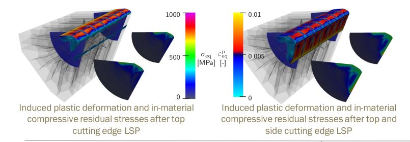
Numerical simulation allows for part- and material-tailored Laser Shock Peening, leading to an increase in LSP applicability and competitiveness.
